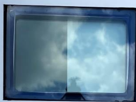
GL-2: VE-1 2M 100 WITH 1/4" FULLY TEMPERED OUTBOARD LITE, 1/2" AIR SPACE, 1/4" FULLY TEMPERED INBOARD LITE ON CLEAR.
